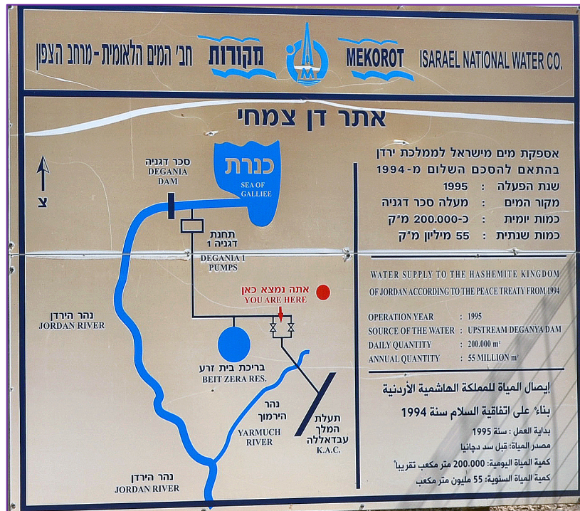
Figure 6.4 Information board at the Beit Zera pumping station showing water supplied by Israel to Jordan, or half of the Yarmouk-Tiberias ‘water swap’. The English part of the sign states: ‘Water Supply to the Hashemite Kingdom of Jordan according to the Peace Treaty from 1994. Operation Year: 1995; Source of the Water: Upstream Deganya Dam; Daily Quantity: 200,000m 3 ; Annual Quantity: 55 million m 3 .’ The figure does not show the rest of the Yarmouk-Tiberias water swap, whereby Israel receives water from the Yarmouk for pumping to the Lake of Tiberias and for local use. Source: Muna Dajani.
